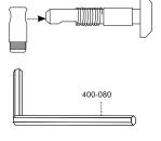
**B.** Install the cross dowels into both ends of the spanner post as shown. Gently tighten the set screw in place with the hex key. (Adjust set screw to move dowel fastener in and out as needed.)
